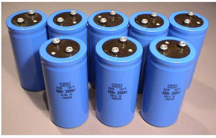
Electrolytic Capacitors, 400V 3900uF
