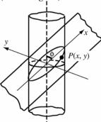
If P(x, y) is a point on C,  $(x \sin \phi)^2 + y^2 = r^2$  where r is the radius of the cylinder. Then
