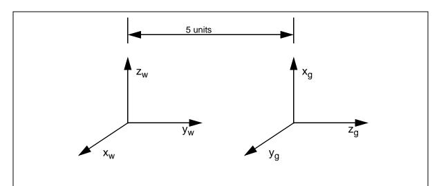
Figure 21. World and gripper coordinate frames for some robot. There are several ways we can think about transforming between the two coordinate frames.
