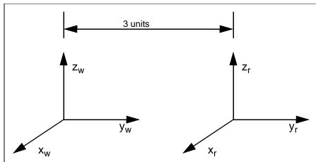
Figure 14. Two coordinate frames, world (w) and robot (r). The origin of the robot frame is located at the point (0,3,0) in world coordinates. Using our new notation, we can represent this as  $\begin{bmatrix} 0 & 3 & 0 & 1 \end{bmatrix}^T$ . The two x axes are parallel, as are the two y and the two z axes. Note that the origin of the world coordinate axes is at  $\begin{bmatrix} 0 & -3 & 0 & 1 \end{bmatrix}^T$  in robot coordinates.
