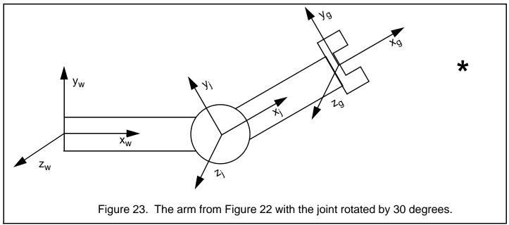
There is one point in this image whose location does not move in any frame as the joint moves. The point located at the very center of the joint (i.e. with Joint coordinates (0,0,0)) is always at world coordinates location (L1, 0, 0), and always at (-L2, 0, 0) in gripper coordinates, no matter how you move the joint.
