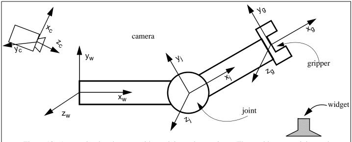
Figure 13. A very simple robot arm with one joint and one gripper. The world, camera, joint, and gripper coordinate frames are indicated.
